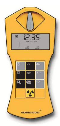
GAMMA-SCOUT® is powered by a 2.7 - 3.7 V lithium thionyl chloride cell. The device will continue functioning until the cell voltage is down to 2.8. When the voltage drops below this value, the battery symbol will appear in the display. The data will be retained, even following a total loss of voltage. The RECHARGEABLE model has a rechargeable battery, which can be recharged via USB (or the power supply unit included with delivery).
